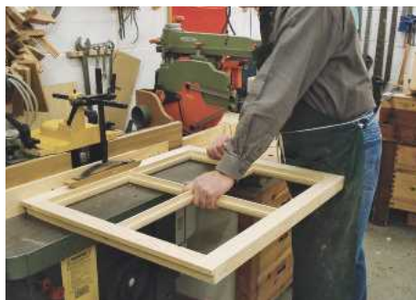
▲ Pic.23 The glazing bars are fitted using halving joints, and the outer edges are moulded...
